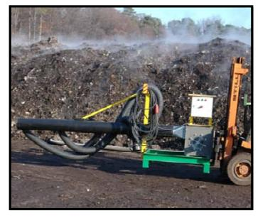
The entire dismantling procedure takes only twenty minutes for a MAF system installed on a 1500 m<sup>3</sup> windrow. The wheel loader now has unhindered access to the windrow.
